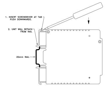
Figure 3.3 — Removal of Unit
